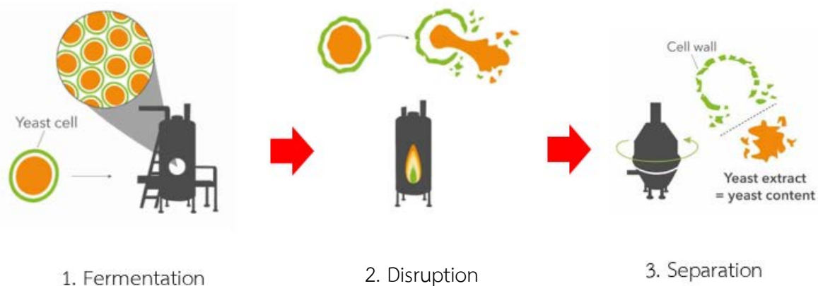
Figure 1 Yeast extracts in general are produced in three steps: fermentation, disruption and separation (17)
